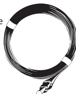
If the centre of the fence system is more than 100m (300 ft) from the Energizer, at least 1 x 2.5mm wire is required. If the centre of the fence system is more than 1km (5/8 mile) from the Energizer, a minimum of 3 x 2.5mm wires or a single High Conductive 2.5mm "PowerWire" is required. Larger fence systems or heavily loaded fence systems with large Energizers may require more wires to adequately transfer the power from the Energizer onto the fence system.
