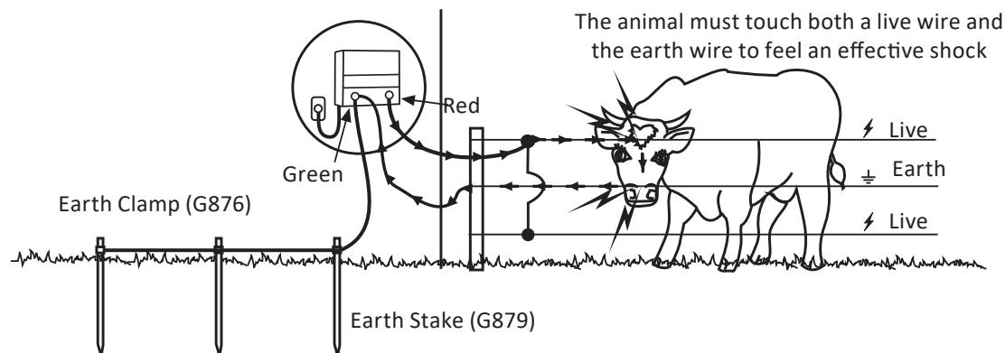
Earth stakes, at least 2m (6ft) long, should be spaced 3m (10ft) apart. Use a minimum of 3 earth stakes.
